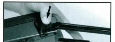
13 - Fold stock back in place by pushing on the release button.
