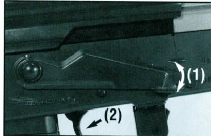
10 - To start shooting, aim at a target, put the selector (1) on one of two low positions (Semi or Full Auto) and pull the trigger. (2)
