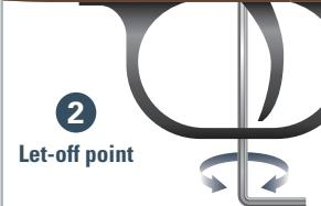
**2. Adjusting the let-off point:** For a heavier let-off point: Turn adjustment screw **2** clockwise. For a lighter let-off point: Turn adjustment screw **2** counterclockwise.
