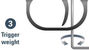
**3. Adjusting trigger weight:** To increase trigger weight: Turn adjustment screw **3** clockwise. To reduce trigger weight: Turn adjustment screw **3** counterclockwise.
