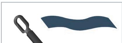
1. Engage the Safety. Attach a piece of cotton fabric to the end of a suitable cleaning rod.
