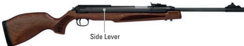
**Note for Model 54:** Mod. 54 is a strong and precise recoilless high power air rifle with fixed barrel and side lever cocking. The elimination of the recoil has been reached through a novel retrograde brake-mechanism. When firing the mechanism is moving 15 mm backward.
