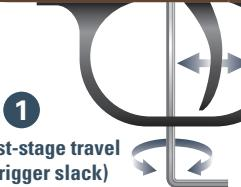
**1. Adjustment of first-stage travel (trigger slack):** To reduce trigger slack: Turn adjustment screw **1** clockwise. To increase trigger slack: Turn adjustment screw **1** counterclockwise.
